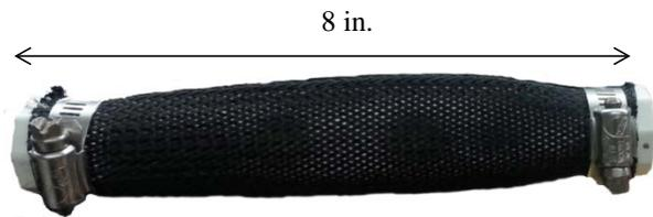
**Figure 2: Final Air muscle Prototype**
