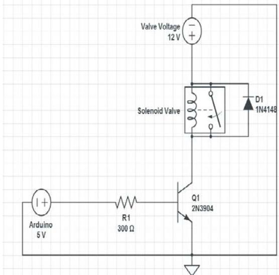
Figure 4: Transistor circuit to control solenoid valve.
